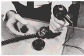
An expert holds a small microphone that can be hidden behind a telephone receiver.
